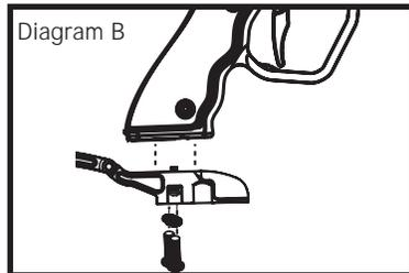
**STEP 4.** Remove field strip pin from the marker. Note: Internal are under pressure, use care.
